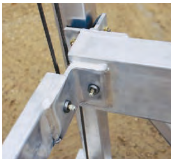
Stainless steel pins with grease zerks.
